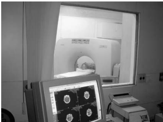
Figure 3. Tomographic device of CEMUPE used to obtain tomographic images of Alderson-Rando phantom.
