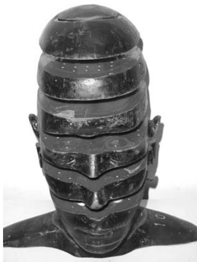
Figure 2. Slices and orifices of Alderson-Rando phantom used to accommodate thermo-luminescent dosimeters.
