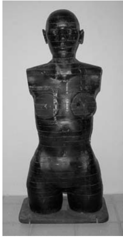
Figure 1. Alderson-Rando female phantom of the Laboratory of Metrology of Ionizing Radiations (LMRI)
