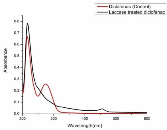
**Figure 4.** UV-Visible absorbance spectra before and after treating with crude laccase.
