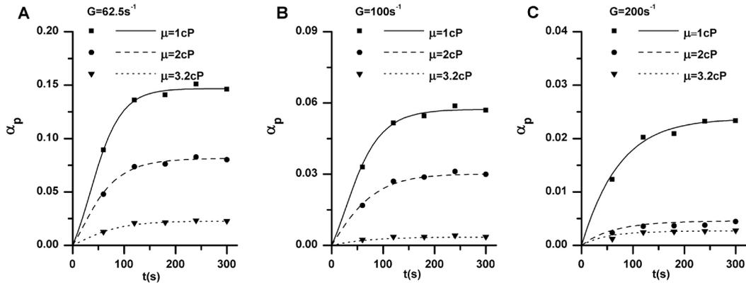
**Figure 5. Results of curve fitting.** The lines are plotted using theoretical formula (16) with parameters taking their best-fit values and dots denote experimental data.  $\mu$  is viscosity.
