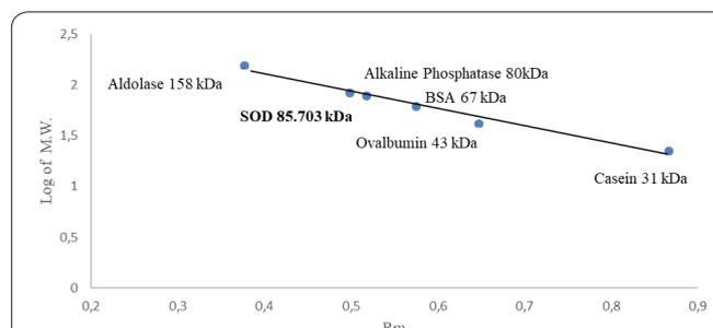
**Figure 6.** Molecular mass of SOD by SDS-PAGE purified from *T. aphylla* L.
