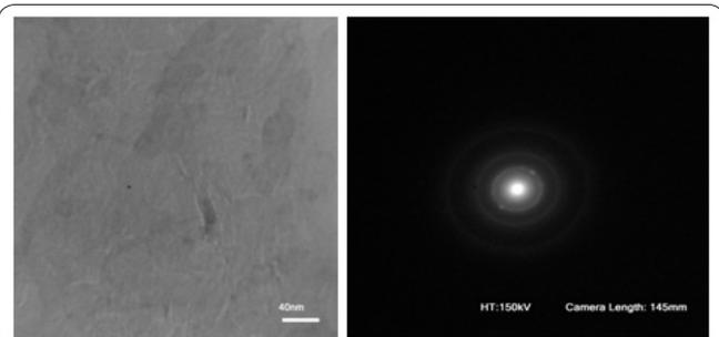
Figure 4. HR-TEM images of Stevia-based carbon dots.
