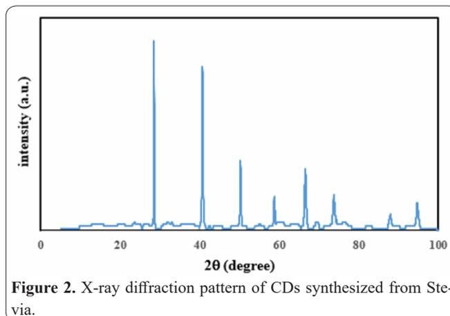
Figure 2. X-ray diffraction pattern of CDs synthesized from Stevia.
