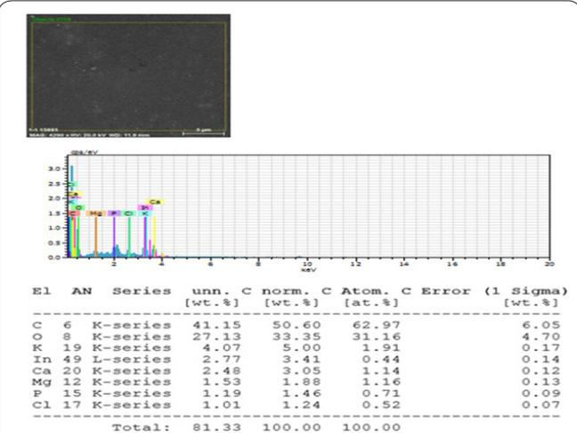
Figure 5. EDS analysis of Stevia-based CDs.
