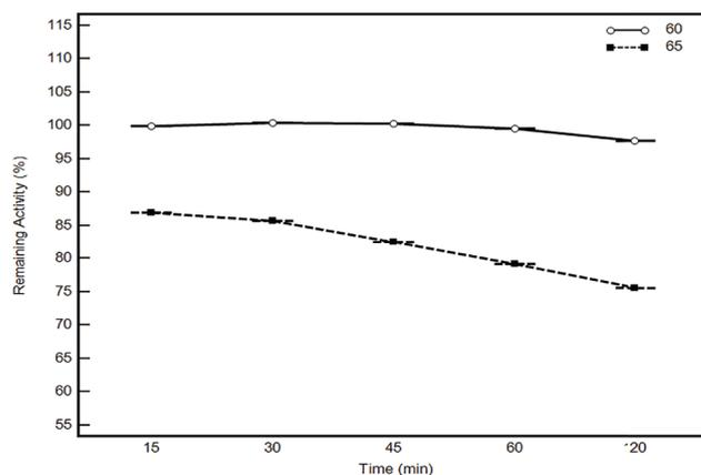
**Figure 7.** Effect of temperature on stability of recombinant  $\beta$ -galactosidase. The purified enzyme was incubated at different temperatures (60 and 65 °C) for different time intervals (15-120 min). The comparisons were made using the unheated crude enzyme activity as 100%. The remaining activity was measured under standard assay conditions.
