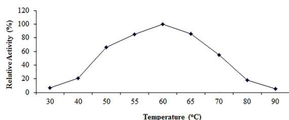
**Figure 6.** Effect of temperature on activity of recombinant  $\beta$ -galactosidase. Optimum temperature was determined under standard assay conditions using *o*NPG at temperatures ranging from 30 to 90 °C. Results represent the means of three experiments, and bars indicate  $\pm$  standard deviation. Absence of bars indicates that errors were smaller than symbols.
