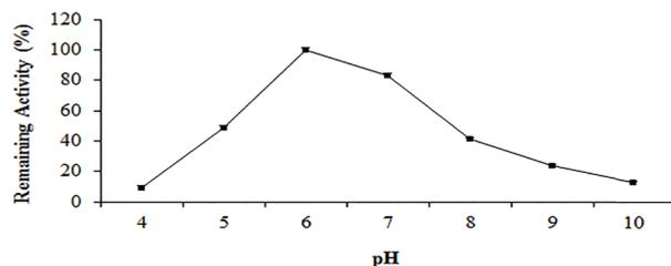
**Figure 5.** pH stability of recombinant  $\beta$ -galactosidase. The purified enzyme was incubated at 60 °C for 1 h in different buffers (sodium citrate buffer pH 4.0-6.0; sodium phosphate buffer pH 7.0–9.0; and glycine-NaOH buffer pH 10.0). The remaining proteolytic activity was measured under standard assay conditions.
